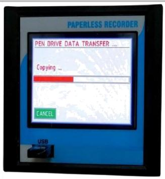
If USB 2.0 drive is not inserted in the drive, an error screen, PEN DRIVE PROBLEM!!! Will be displayed.
